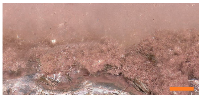
Figure 2. High-resolution imaging of the K-rich NaK alloy after 3 mAh cm -2 of charge has been passed with a 2 mA cm -2 charge rate. Scale bar is 250 μm.
