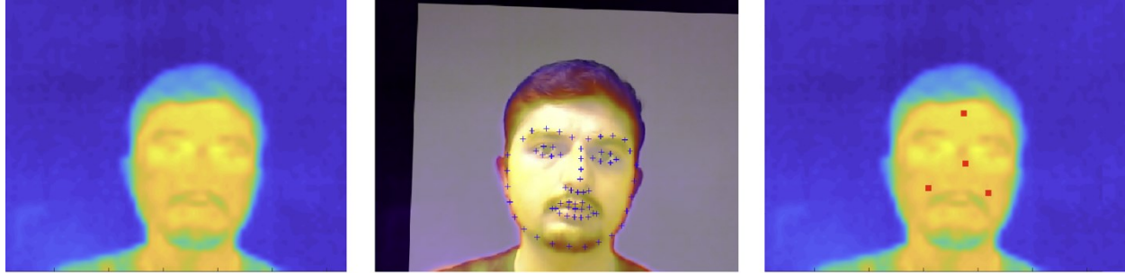
Figure 4: Steps of temperature extraction from different ROIs in thermal images. From left to right: thermal image, landmark detection using RGB image overlaid on thermal image, identified ROIs on thermal image.
