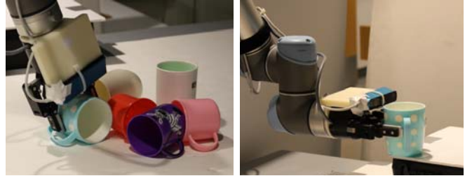
Fig. 1. Pick-place problem considered in this paper. The robot must grasp and place an object in a desired pose without prior knowledge of its shape.
