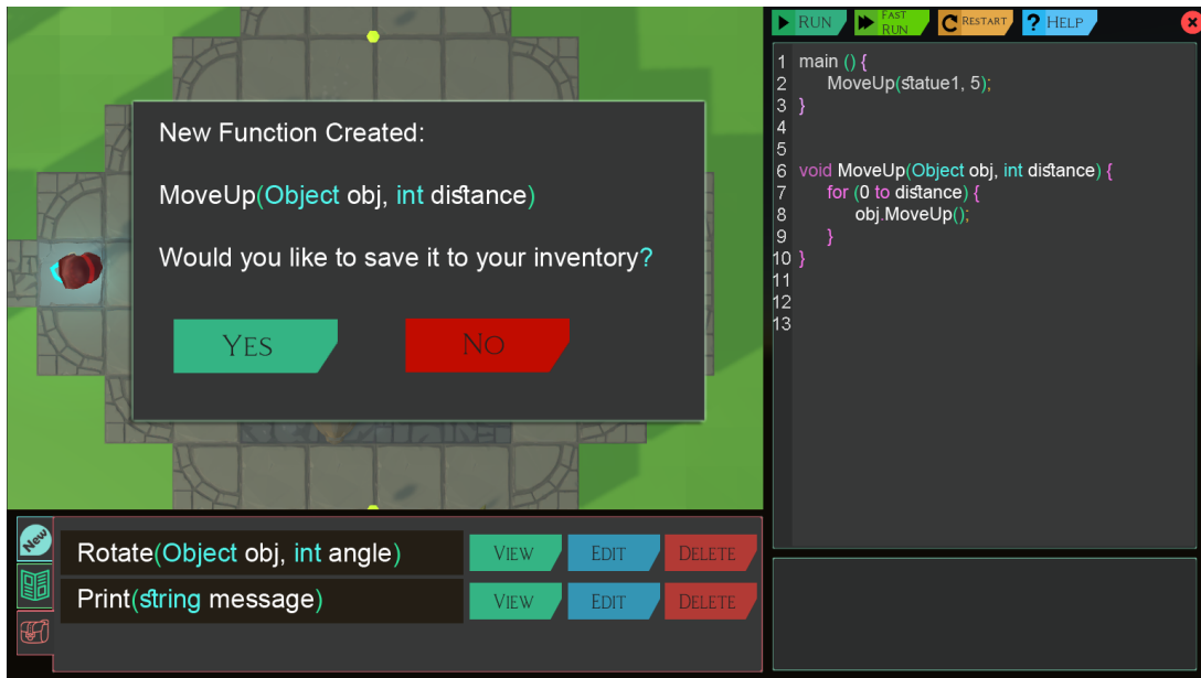
Figure 3: Design of the library/inventory system: After running a correct program, the player is prompted whether they would like to save new functions they created into their inventory. The bottom left part, shows previous functions that players have saved, they can be viewed, edited, or deleted.
