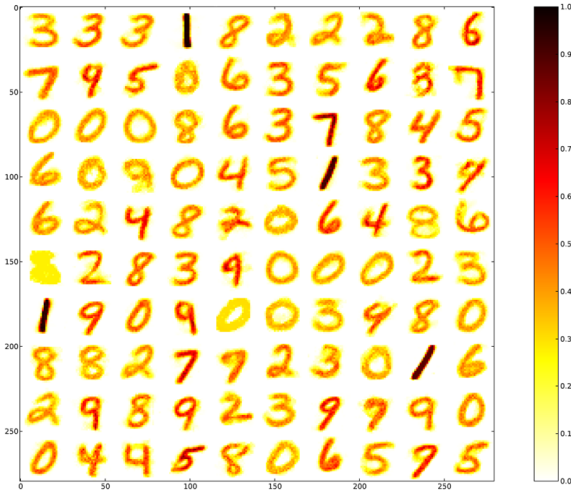
Fig. 8: Weights of the excitatory synapses after only 6000 training samples are provided. Most set of synapses already settled to a clear prototypical input. The scale on the right hand side represents the weight strength. The darker a pixel is, the stronger the synaptic weight.
