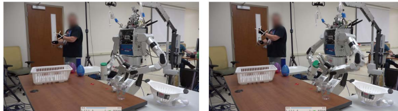
Figure 5: A novice user executing various sub-tasks from Study 1. The sub-tasks in Study 1 followed a breakfast-making theme, matching our motivated use-case of our bimanual shared-control method being used in remote home-care or telenursing scenarios.
