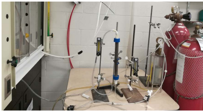
Figure 1: Column experimental setup (with humid gas): (a) Schematic; and (b) Photograph.
