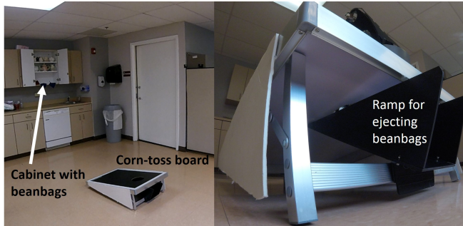
Fig. 7: Study setup at the PACE center (left). The game bean bags were initially placed in the cabinet. A modification ramp was added under the board so that bean bags would be ejected when scored, facilitating its retrieval by the robot.
