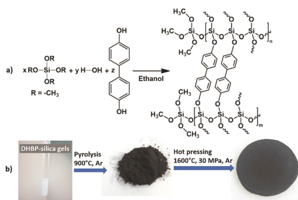
Fig. 2 Sol-gel synthesis of orthosilicate-based single-source precursors containing large, aromatic substituents (a); their ceramization at 900 °C and uniaxial hot pressing at 1600 °C under an Ar atmosphere to produce monolithic ceramic samples (b).
