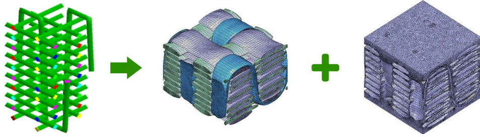
Figure 1. Unit cell of one-by-one orthogonal composite panel: from the initial schematics of the reinforcement for DFMA simulations to the finite element mesh (reinforcement + matrix) in MSC Marc Mentat.
