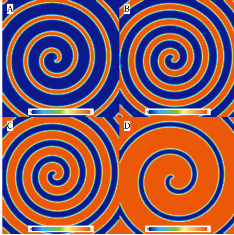
Fig. 11. Spiral wave in the Barkley model initiated when the parameters of the Eq. (9) were set to a = 0.5 , b = 0.04 , and \epsilon = 0.02 (panel A). Then, parameter a of the model was slowly and interactively changed to 0.8, 1.0, and 1.2 from B to D. Note how the wavelength increases as a is increased.
