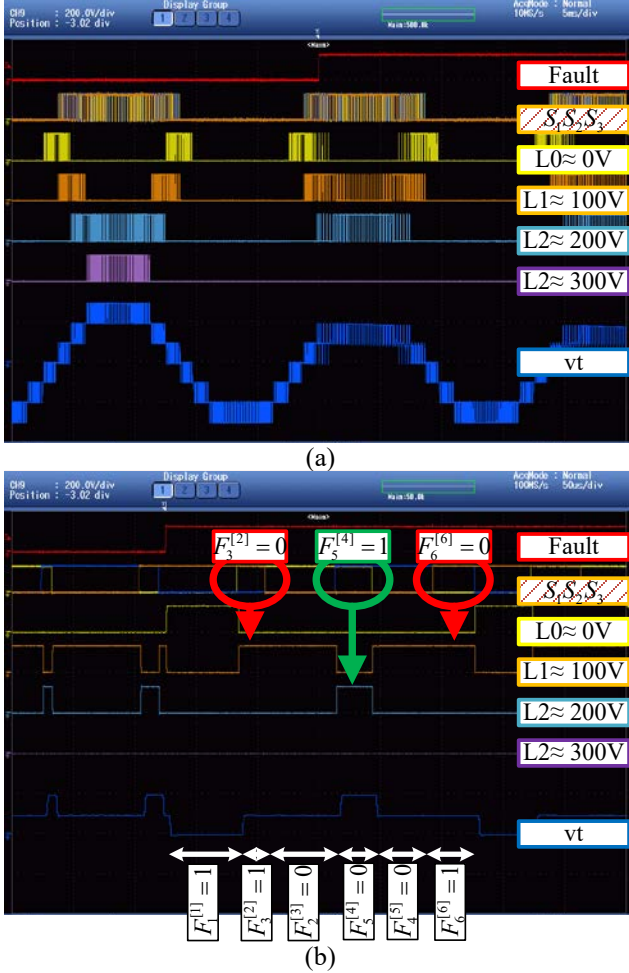
Fig. 9. OC-fault on S_3 (Top-Rail) when 100V < v_m < 200V ; (a) all signals for positive modulation (b) Zoomed signals \vec{F} = [F_3^{[1]}, F_5^{[3]}, F_6^{[5]}] = [101] .
