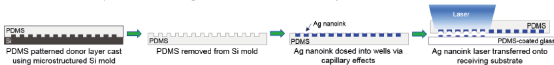
Figure 1. Schematic depicting fabrication of PDMS patterned donor layer and subsequent laser transfer of Ag nanoink onto receiving substrate.
