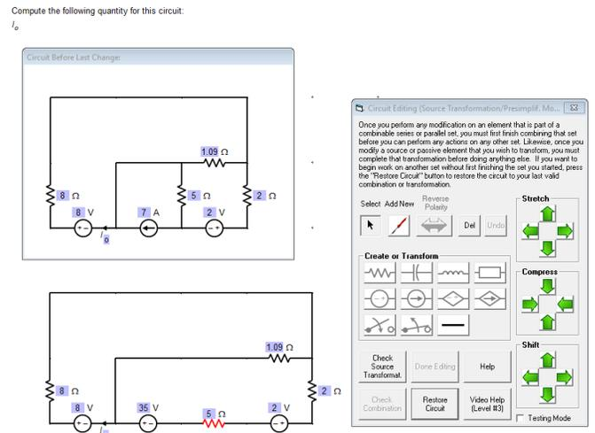
Fig. 2. Source transformation example. User has just transformed a 7 A source in parallel with an 8 Ω resistor into a 35 V source in series with the same resistor (having “stretched the circuit horizontally to make room on the grid), and is about to check that action in the circuit editor. The last valid circuit is always shown in the window above for easy reference.
