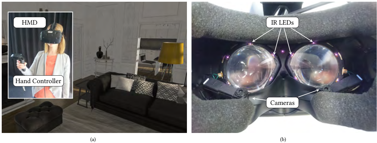
Fig. 3. A participant of the experiment wearing the HTC Vive HMD and a hand-controller (inset) and the virtual environment of the experiment, which is an architectural visualization of a living room (a). Inside the HMD, the Pupil Labs eye tracking device was integrated (b). It consists of several infrared LEDs to illuminate the eyes and two cameras to enable stereoscopic tracking.
