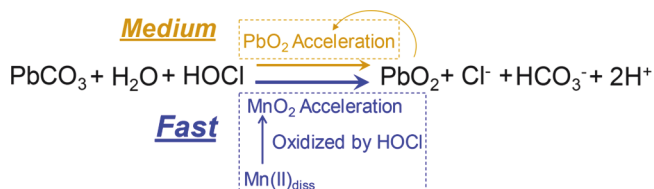
Figure 2. Conceptual model of \text{PbO}_2 formation from cerussite considering \text{PbO}_2 autocatalytic and \text{MnO}_2 catalytic effects. Both the hypochlorite ion and hypochlorous acid can oxidize Pb(II) to Pb(IV), and only the hypochlorite ion is shown here for the sake of simplicity.
