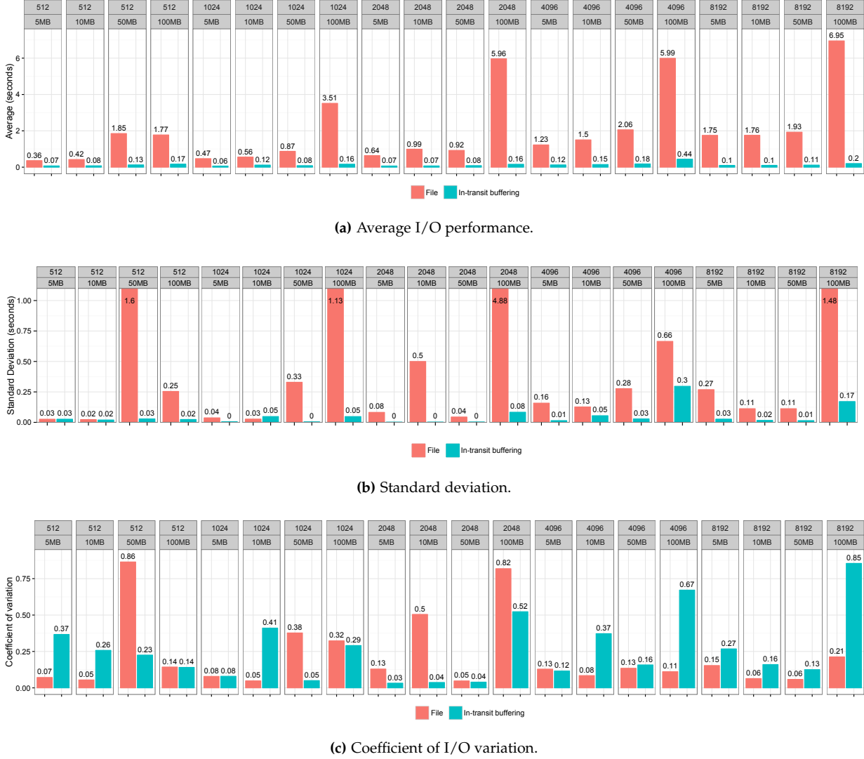
Fig. 16: Performance comparison between file I/O and in-transit buffering. We conducted experiments over a few weeks of time period with different data volumes (from 5 MB up to 100 MB of data per process) over different scales, ranging from 512 up to 8,192 nodes. All tests were performed on Titan.
