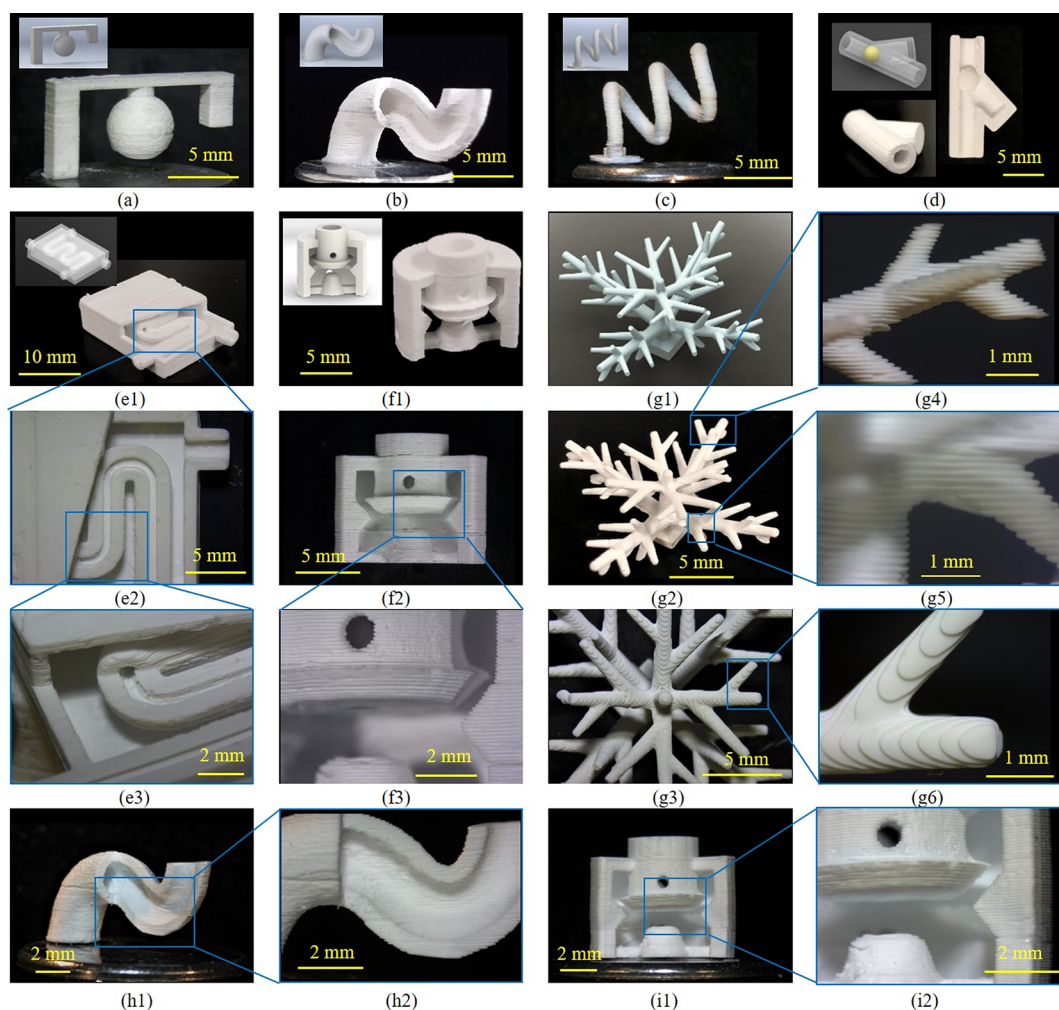
Figure 5. Fabrication results via the SEPS process: (a) a structure with an overhanging ball and cube; (b) a tube with an inner overhanging chamber; (c) a spring structure printed with an upward slope angle; (d) a ball check valve with an inner chamber and a movable ball inside printed without assembly; (e) a heat exchanger with an inner chamber and overhanging hollow pipeline (e1–e3); (f) a combustion chamber with overhanging nozzles (f1–f3); (g) a CAD model of a treelike structure (g1) and the printed treelike structure and its microstructures (g2–g6); (h1, h2) the sintered overhanging tube; (i1, i2) the sintered combustion chamber.
