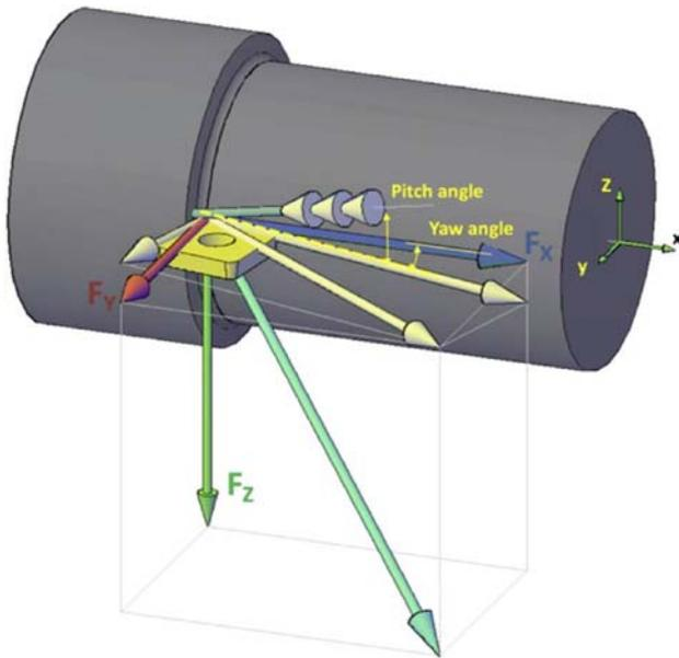
Fig. 5 The cutting forces measured and the orientation of MQL nozzle in turning center
