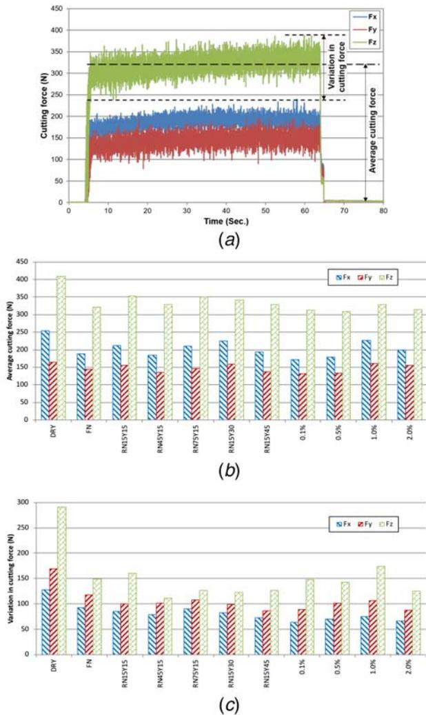
**Fig. 7** Cutting forces in  $x$ ,  $y$ , and  $z$  directions under various conditions: (a) force signals from dynamometer, (b) average cutting forces, and (c) variation in cutting force
