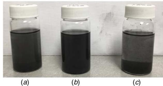
Fig. 3 Stability in mixtures of oil: (a) 0.1, (b) 0.5, and (c) 1.0 wt% xGnP M5 after 72 h
