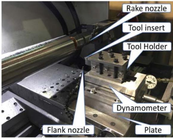
Fig. 4 Experimental setup
