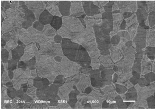
Fig. 1 Microstructure of Ti-6Al-4 V in the STA condition
