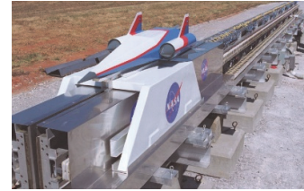
Fig. 8. Electromagnetic river demonstrator for maglev launch assist built at NASA's Marshall space flight center in Huntsville, Alabama [79]
