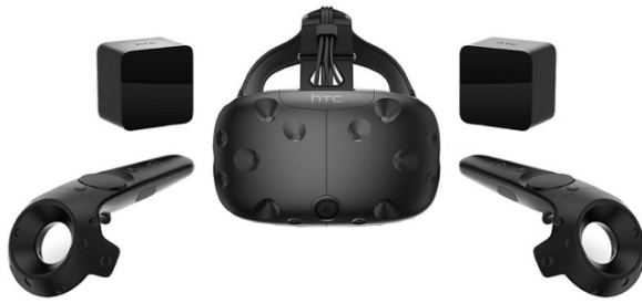
Figure 1: The HTC Vive system, which contains a headset, two handheld controllers, and two motion tracking sensors.
