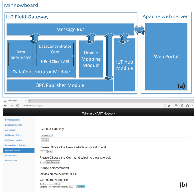
Fig. 2: (a) Software architecture of the IIoT field gateway (IIoT-FG); (b) web portal for remote access and network/device configuration.
