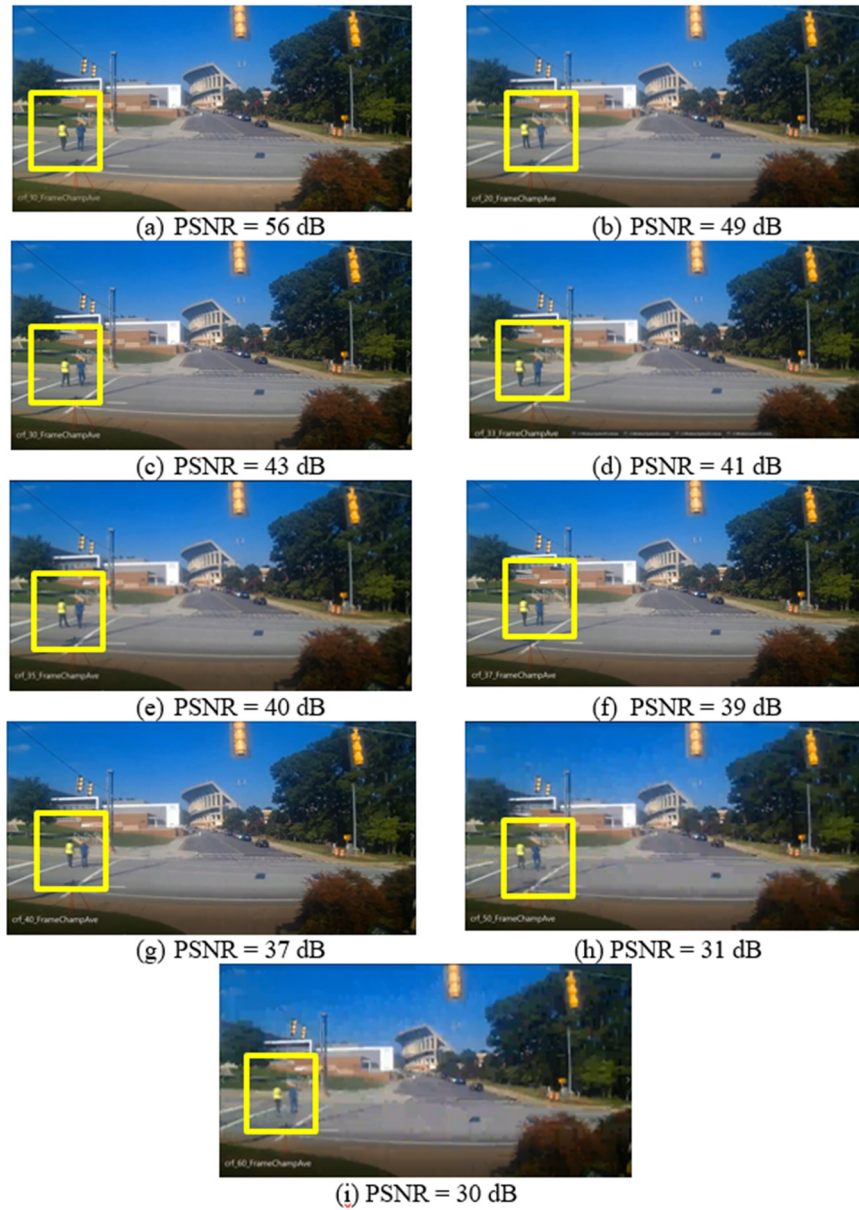
Figure 4. Compressed images from the field-collected data using increasing levels of video compression and different PSNR values.
