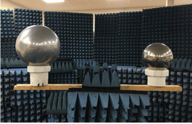
Fig. 12. Two reflecting spherical targets used as the 2-D scene.
