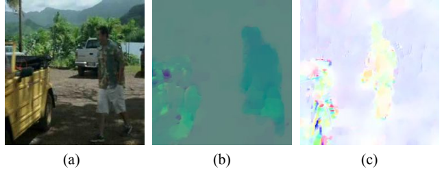
Figure 1: Comparing the results of (b) TVL-1 and (c) our learned flow when applied to RGB images. Our layer is able to capture similar motion information to TVL-1. However, compared to TVL-1, our layer is faster, is learnable, and can be applied directly to any intermediate CNN feature maps. With the representation flow layer, optical flow pre-extraction is no longer needed and a single-stream CNN design becomes possible.
