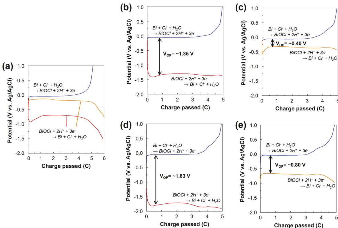
**Figure 3.** Potential–charge plots for Bi and BiOCl electrodes measured vs a Ag/AgCl RE at  $\pm 1$  mA  $\text{cm}^{-2}$  obtained (a) in an undivided cell as half-cell reactions, (b) in a two-compartment Bi(60 mM NaCl)/BiOCl(60 mM NaCl) cell, (c) in a two-compartment Bi(60 mM NaCl)/BiOCl(65 mM HCl) cell, (d) in a three-compartment Bi(60 mM NaCl)/60 mM NaCl/BiOCl(60 mM NaCl) cell, and (e) in a three-compartment Bi(60 mM NaCl)/60 mM NaCl/BiOCl(65 mM HCl) cell.
