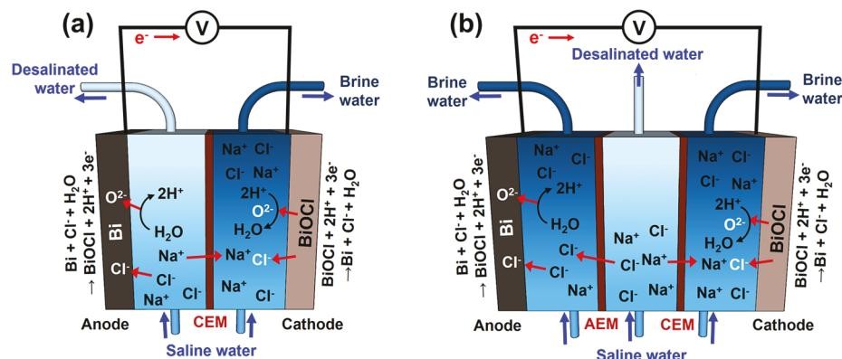
Figure 2. Cell configurations and operating schemes of (a) two- and (b) three-compartment Bi/BiOCl ED cells for desalination.
