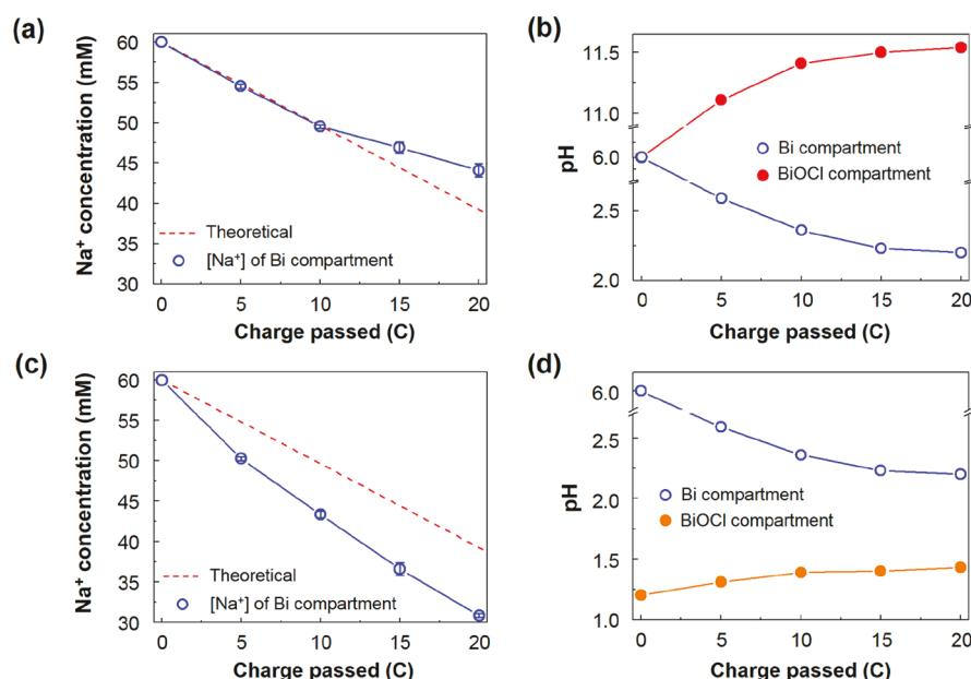
**Figure 4.** (a) Change in  $\text{Na}^+$  concentration in the Bi compartment and (b) change in pH in Bi and BiOCl compartments of the Bi(60 mM NaCl)/BiOCl(60 mM NaCl) cell operated at  $1 \text{ mA cm}^{-2}$ ; (c) change in  $\text{Na}^+$  concentration in the Bi compartment and (b) change in pH in Bi and BiOCl compartments of the Bi(60 mM NaCl)/BiOCl(65 mM HCl) cell operated at  $1 \text{ mA cm}^{-2}$ .
