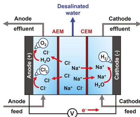
Figure 1. Scheme for desalination performed by a conventional ED cell.
