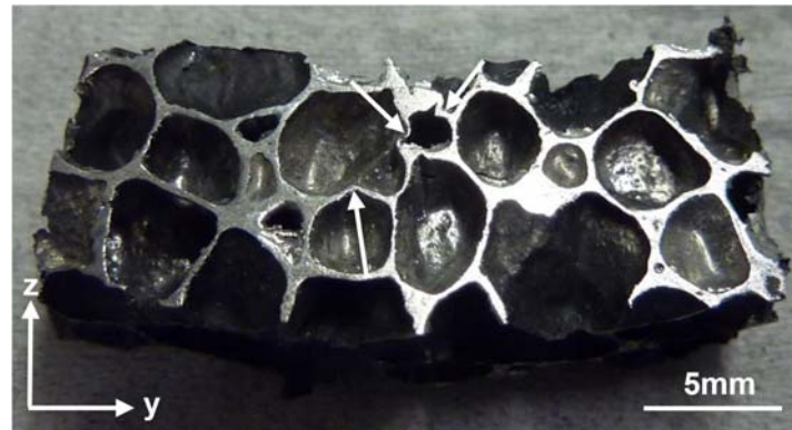
Figure 4 Cross-section of a foam specimen after 5 laser scans at a power of 180 W and a scan speed of 10 mm/s (see online version for colours)
