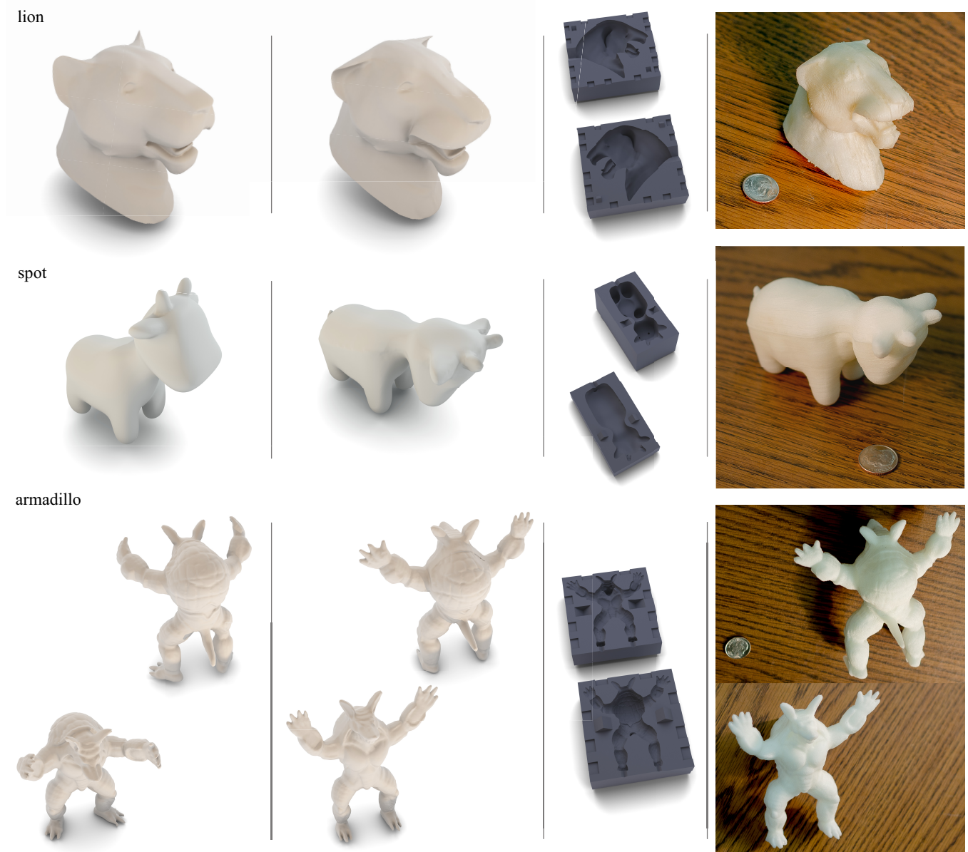
Fig. 17. Multiple casts fabricated via our method. The far-left column shows the input mesh; the left column shows the result mesh after applying our method; the right column shows the 3D-printed molds; the far right column shows the foam casts (dime for scale). The shapes undergo large deformations to become castable, but remain close to the input in terms of character.
