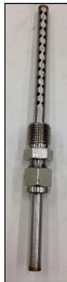
Figure 18 Designed diffuser to disperse O 2 into the exhaust stream
