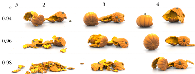
Fig. 16. NACC Parameters. The NACC parameters \alpha and \beta are shown to strongly control fracture behavior, giving significant artistic control.
