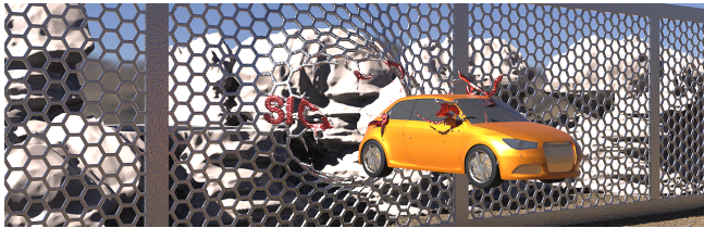
Fig. 18. Fence Smash. A getaway car smashes through a metal fence leaving intricate ductile debris and demonstrating the results attainable through pairing von Mises plasticity with PFF-MPM ( \tau_y = 35 ).
