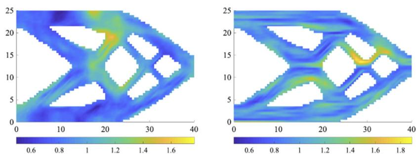
**Fig. 5** Posterior configurations obtained for the isotropic (left) and anisotropic (right) cases for  $K = 3$
