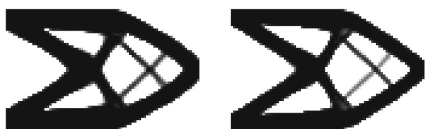
**Fig. 6** Difference between the optimized solutions generated with locally isotropic (left) and anisotropic (right) kernels and the deterministic solution
