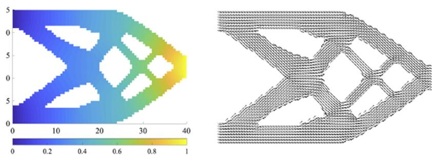
**Fig. 4** One sample of the Young's modulus random field obtained for the isotropic (left) and anisotropic (right) cases
