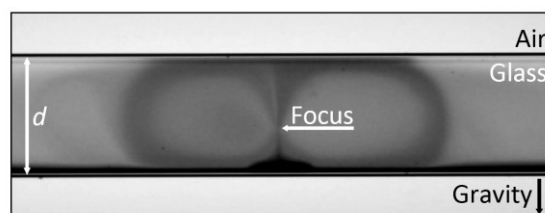
Figure 6 A photograph of a glass capillary in which gold nanorods have been driven into motion by thermophoresis resulting in a convection pattern. The laser beam is centered on the d = 2.00 \text{ mm} wide window and is directed into the page.
