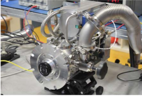
Fig. 1. Left: photograph of the MIRC-X C-RED ONE. Right: scheme of the experimental setup. 1: H band single-mode fiber fed by a white-light source; 2: dispersion prism; 3: camera cold stop and baffle; 4: low pass cold filter; 5: detector.
