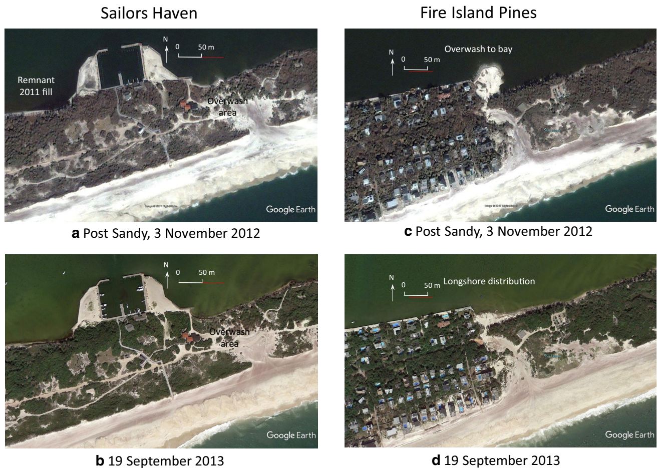
Fig. 9 Overwash areas created during Hurricane Sandy east of Sailors Haven ( a and b ) and Fire Island Pines ( c and d )
