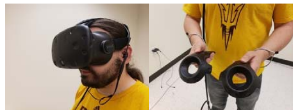
Figure 2. Close-up of HTC Vive equipment. Left: Headset and earbuds. Right: Vive controllers with vibrotactile feedback capabilities to simulate feeling the rumble of the crowd.
