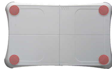
Figure 2: Positions of the pressure sensors located inside of the Wii Balance Board.
