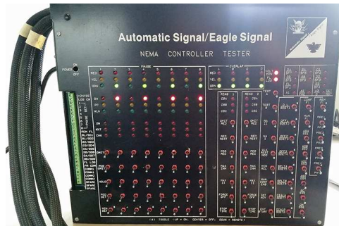
Fig. 6: All-direction green lights being displayed on traffic signal test equipment. The left 4 green LEDs represent the through directions of travel at an intersection while the right 4 green LEDs represent the corresponding left-turn lanes.
