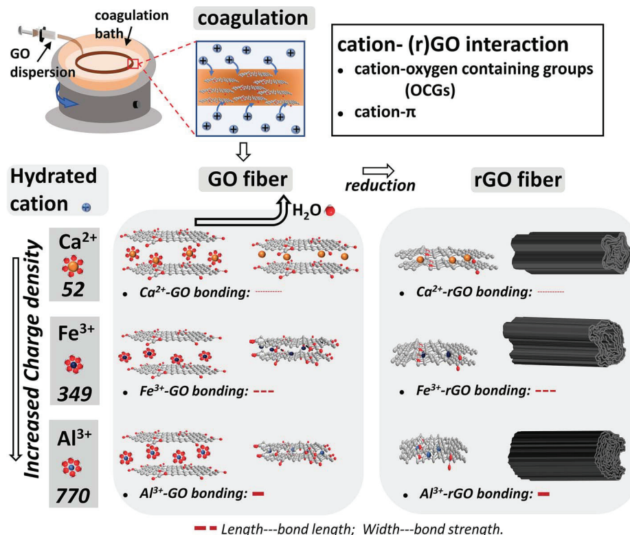
Fig. 1 Schematic illustration of the formation of rGO fibers from divalent and trivalent cations in coagulation baths, respectively. After solvent evaporation and chemical reduction, rGO fibers with different cation cross-linking resulted in dramatically different morphologies.
