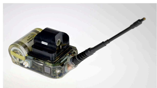
FIGURE 2 | A CTD-SRDL tag, featuring a miniaturized CTD on top of the core unit, with the microcontroller below, the wet/dry sensor on the frontside, the battery on the rear, and the Argos antenna pointing forward.
