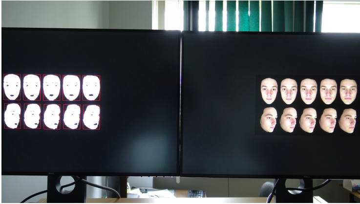
Fig. 6. Working system. Right screen – input image. Left screen – CCA/CCL result.
