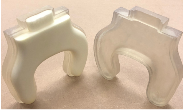
Fig. 2. 3D printed mold and cast foam planar gripper.
