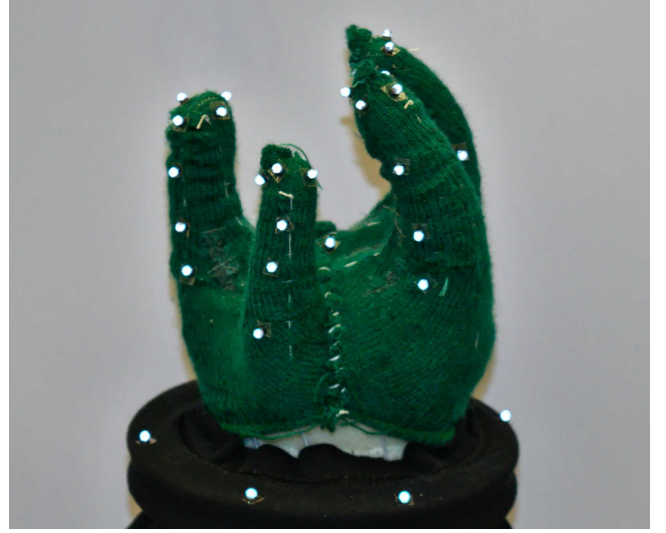
Fig. 5. Four-fingered hand with Vicon markers.
