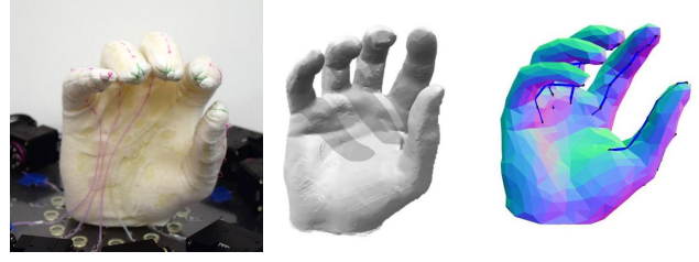
Fig. 8. Anthropomorphic foam hand prototype in its rest pose. Left) physical foam hand prototype, Middle) Scan of the prototype, Right) Finite element mesh used in simulation.
