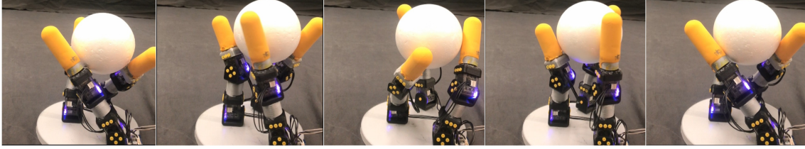
Fig. 3. To demonstrate the feasibility of our designs, we fabricated a hand with 3d-printed parts scaled with regard to the embedded motors. This particular design is meant to rotate a 4 inch diameter ball 180 degrees either way.
