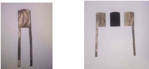
Figure 1. Assembled sensor (left) and layers (right)
