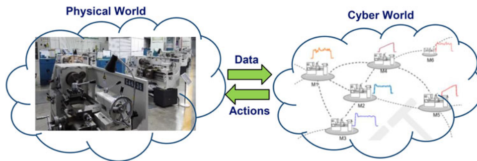
Figure 6. Cyber-physical manufacturing systems. The manufacturing enterprise is reflected in the cyberspace through data, and analytics run in the cyberspace feed the actions back to the physical world.
