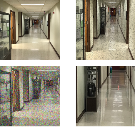
Fig. 2: An illustration of randomly chosen augmentation strategies. From left to right are original, random cropping and pixel dropout, additive Gaussian noise and contrast changing, and more aggressive random cropping.
