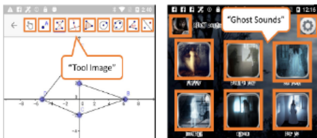
Figure 4: Two example app interfaces with duplicate label errors on image-based buttons. (left) The Clickable Image buttons for drawing different types of figures in a graphing app are all labeled "Tool Image." (right) In the Ghost Sounds app, all of the Clickable Image buttons for playing different ghost sounds as well as the settings and home button are labeled only "Ghost Sounds."
