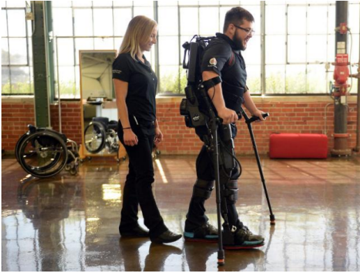
Fig. 3. Ekso Bionics exoskeleton, EksoGT TM , used for data collection. We use two sets of its sensors in this study: hip and knee encoders to generate kinematics-based dynamical models using the NCD algorithm, and foot-mounted pressure sensors at the heel and toe to validate our models against ground-contact events after partitioning.
