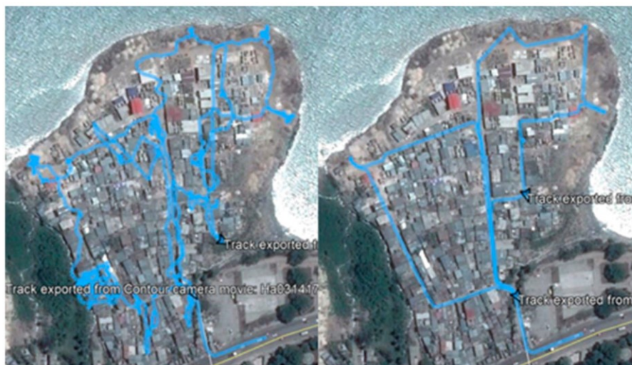
Figure 3. Maps displaying GPS (global positioning system) path corrections in the EC study area. In each image, the blue line shows the walking path connecting test locations. The path on the left is the GPS extracted from the camera. The path on the right has been corrected.
