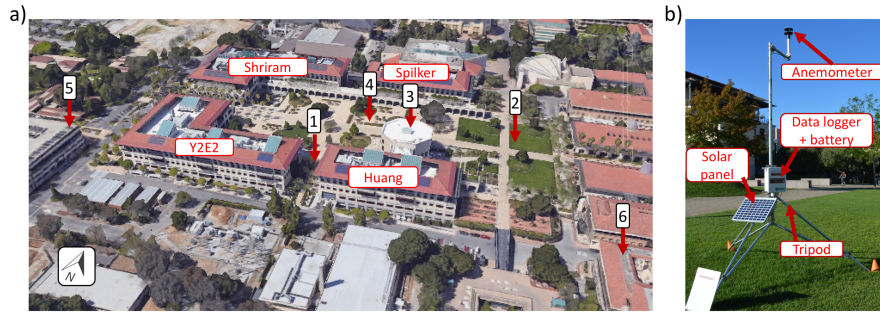
Figure 2: a) Locations of the sonic anemometers within the SEQ b) Example of an anemometer deployed during the experimental campaign.
